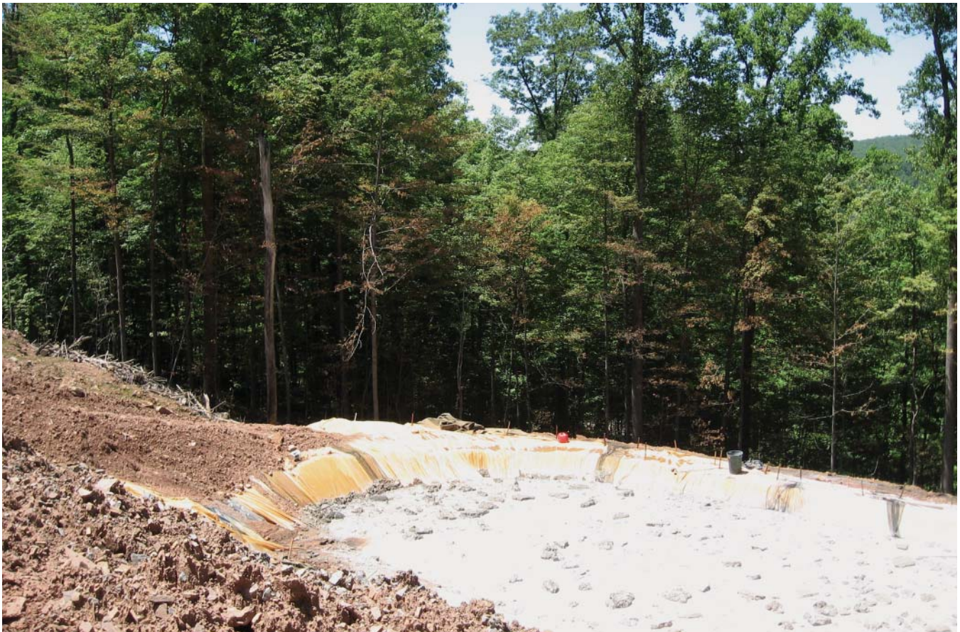
Figure 4. —Foliar injury of trees damaged by aerial release of drilling fluids on May 29, 2008, from the B800 well. Pit containing drilling fluids is shown in the foreground. Photo taken June 11, 2008. Photo by U.S. Forest Service.
