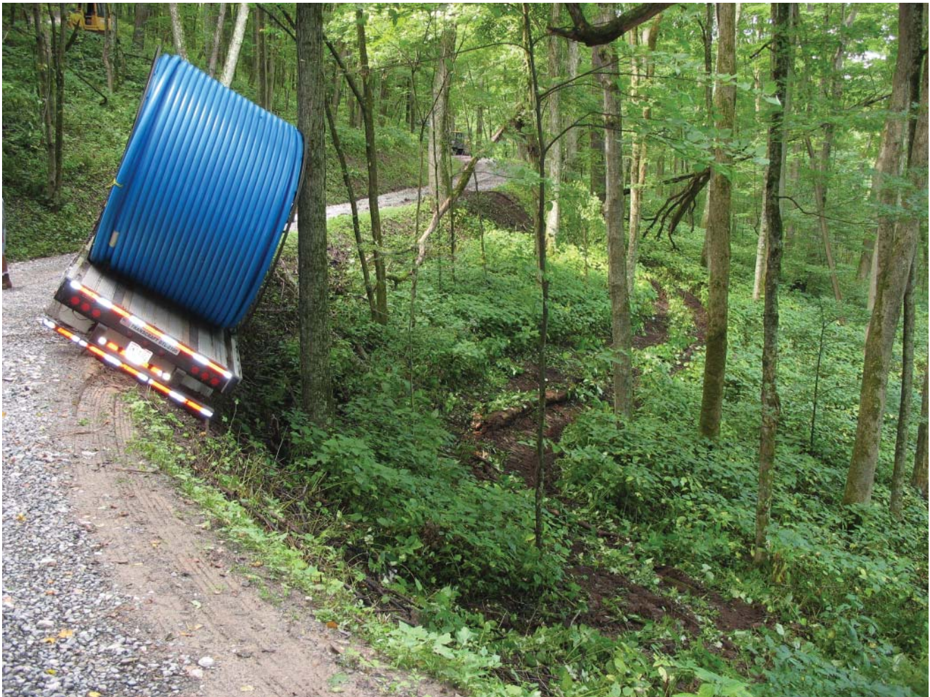
Figure 12. —Biological Control Area, Fernow Experimental Forest, showing damage from truck hauling gas pipeline and from the bulldozer used in an attempt to push the truck back onto the road surface. Photo taken August 13, 2008. Photo by U.S. Forest Service.
